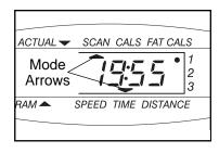
the scan mode is selected, the console will display the speed, time, distance, fat calories, and calories modes, for five seconds each, in a repeating cycle.
